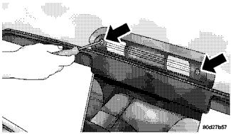
2. Separate the connector holding the housing and wiring harness to the body.
